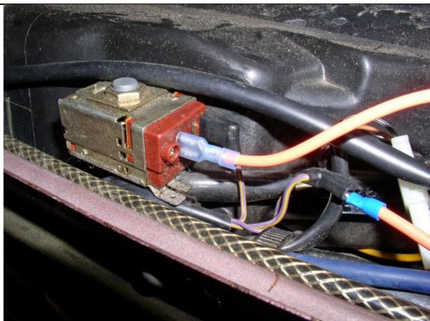
Slide the protected female connector on the freeze switch terminal.
