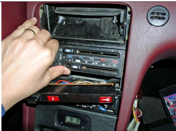
I finished pressing the control unit into place making sure it was not getting hung up on any wiring in the console. As an option, you can remove the console side cover on the right (passenger) side to monitor the re-installation of the head unit. Although it was not required, I removed it anyway because I wanted to see the clearances between the relay and the foot well vacuum actuator arm.
