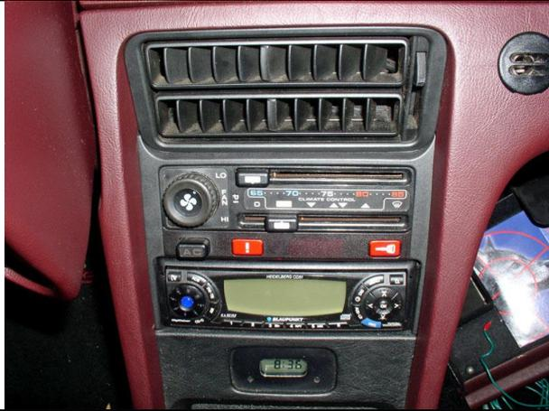
This completes the interior install. You can test the head unit operation once again now that it's secured. Re-install the console side cover if you removed it.
