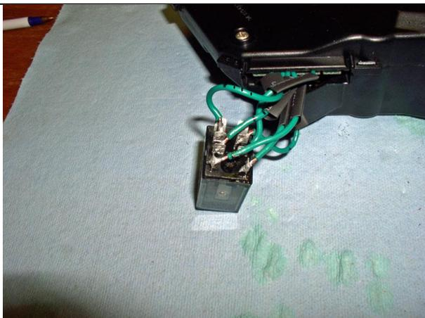
The back side of the new relay is marked with pin numbers corresponding to the schematic on the top of its case. Using the pin mapping worked out earlier, solder the corresponding wire numbers to their mapped tab on the new relay (e.g., wire #4 goes to tab #3 on the relay, wire #1 goes to tab #4 on the relay, etc.).
