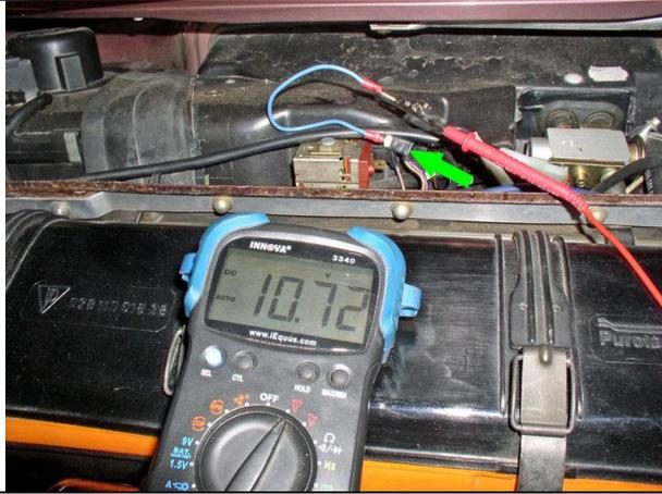
...and inserted the spade into the 2-wire connector and turned on the ignition but did not start the car and pressed the A/C button while the lower slider bar was not set to "off". I received battery voltage. I ran the same test with the car running and received 13.5 volts. So I concluded power was getting to the freeze switch but I could not determine if it had sufficient amperage to drive the magnetic clutch.
