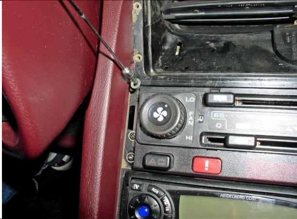
When removing the small screws and washers, consider using a magnetic pick-up tool to extract the screws so they don't fall into an abyss and get lost.
