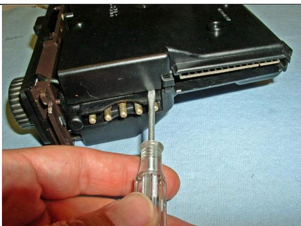
Begin prying the two halves of the head unit covers apart. I started with the side with the used electric ports. It has just one small locking tab that easily separates with the use of a small flat blade screwdriver.
