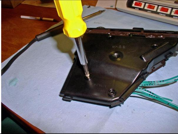
Install the back plate of the head unit and tighten the 4 screws. Ensure the wires are all laying flat against the PC board while installing the cover.
