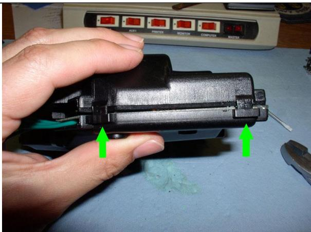
Align the locking tabs and press the two halves together so all locking tabs are engaged.
