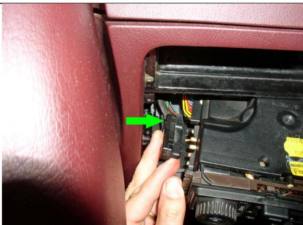
As you are pulling the head unit out, remove the forward harness connector as shown below. You may need to use a flat blade screwdriver to pry the connector loose at first.
