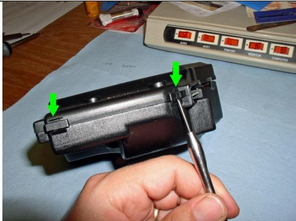
The two rear tabs would not separate so easily, I discovered. Therefore, I had to find a really small screwdriver and I pushed it directly up into the locking tab then levered the screwdriver upward to disengage the lock tab.
