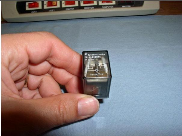
Next, prepare a clean work surface to disassemble the head unit and perform the repairs. Here's a picture of the new replacement relay I purchased from Radio Shack. This relay costs about \$8.00.
