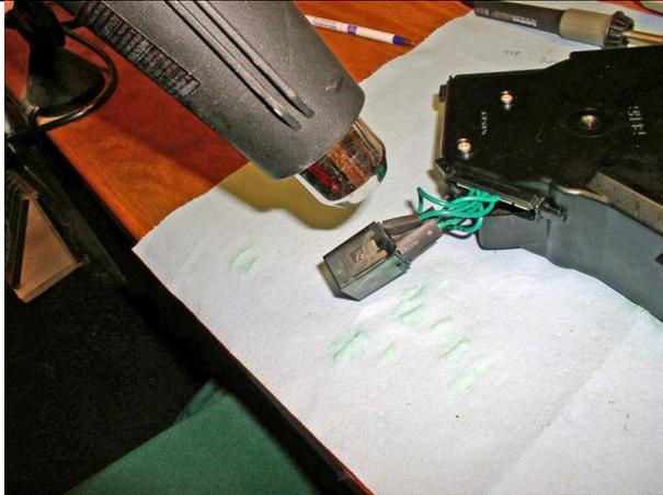
Using a heat gun or hair dryer, heat the shrink tubing.
