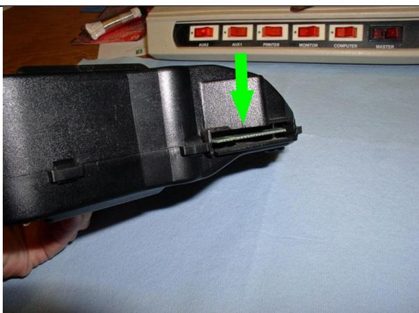
I followed Dr Bob's recommended location for externally mounting the new relay as well as the area for the wire leads to emerge from the inside of the head unit. This area is at the unused port at the back of the unit depicted by the green arrow below.
