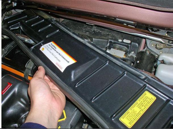
Ensure all jumpers are removed and replace the plastic rain cover.
