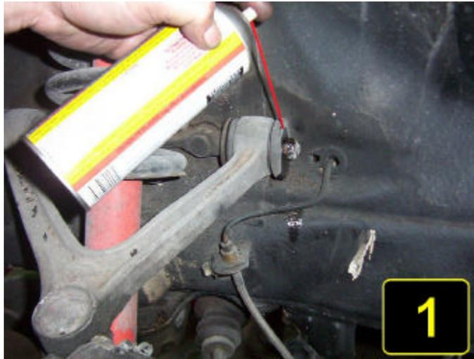
We recommend that you break torque on the 19mm nuts on the ends of the upper A-Arm Spindle now, while the Upper A-Arm is in the car. This will save you a lot of work later. Do not remove the nuts at this time, just break them loose.
