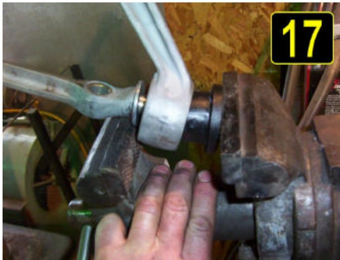
Picture #17. Use the vise and start the other side of the polyurethane bushing into position.
